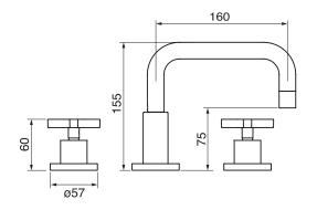
Includes push drain 1.5 GPM (5.7 L/min.)
