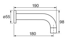
25mm diameter 1/2" male NPT inlet Sliding flange
