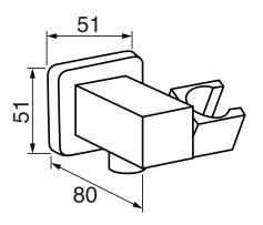
Adjustable shower hook Built in wall supply Brass, chrome plated 1/2" male NPT inlet Sliding flange
