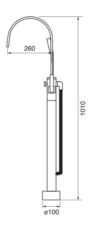
Includes rough-in 5 GPM (18.9 L/min.)
