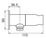
Round metal sprayer with round flange Easy clean nozzles 1/2" male NPT inlet Turn mounting hook for on-off Easy slide installation
