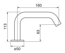
Includes push drain 1.5 GPM (5.7 L/min.)
