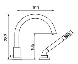
5 GPM (18.9 L/min.)
