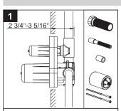
This valve is designed to fit into a wall that is 2 3/4" to 3 5/16" from finished wall to the back of the valve. If necessary extensions can be purchased separatley.
