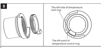
This thermostatic valve has been preset at the factory to deliver water at a maximum of  $120^{\circ}\text{F}$ . If the temperature limit ring is not in the positon of  $120^{\circ}\text{F}$ , please take it out, and having the left side of temperature limit ring get align with the 4th point of temperature control ring( see the arrow in red ), and then re-assembled.
