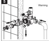
Warning: If soldering is required for any connection remove the cartridge and check valve assemblies before soldering.
