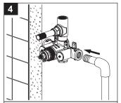
Connect valve body 3/4-NPT inlets to water supplies using the proper fittings. Warning: This valve does not offer a back-to-back installation option.
