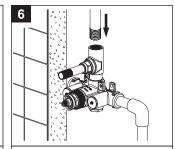
Connect top outlet with proper fittings.Note: it is suggested that you anchor all water lines.
