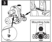
Using mounting holes secure the valve making sure the "UP" label outlet is on top. Facing the valve, the hot supply must be on the left and the cold on the right.
